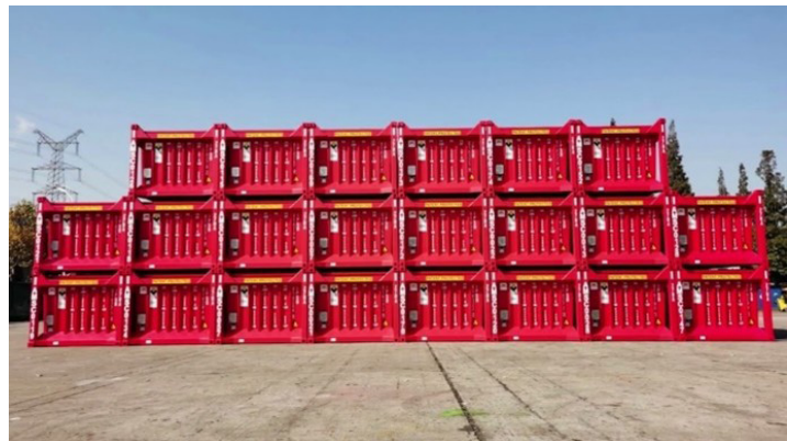
FIGURE 3-2: "ROTAINERS" IN STACKED STORAGE (5-HIGH CAPABLE)
